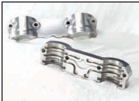
Figure 2. Aluminum camshaft bearing cap
