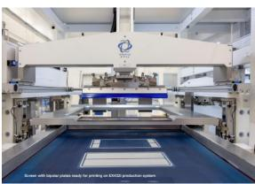
The additive screen-printing process for forming 3D green body parts uses mature precision screen-printing techniques that have been widely used in the printed circuit, semi-conductor, and other high volume sectors for decades.
